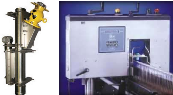
Fig 21 Some examples of sealed radioactive sources used for industrial gauging. The device on the left is an in-line density gauge and is contained in a bright yellow steel-encased lead shield. The item on the right uses a 241 Am source to check product compliance in the beverage industry
