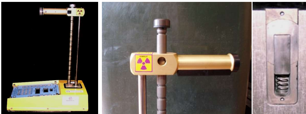
Fig 25 the picture on the left shows an NDM in “SAFE” position while the picture in the middle is the “BACKSCATTER” position and the source is therefore unshielded at this point. The picture on the right shows the sliding tungsten shield assembly once the bottom plate has been removed.
