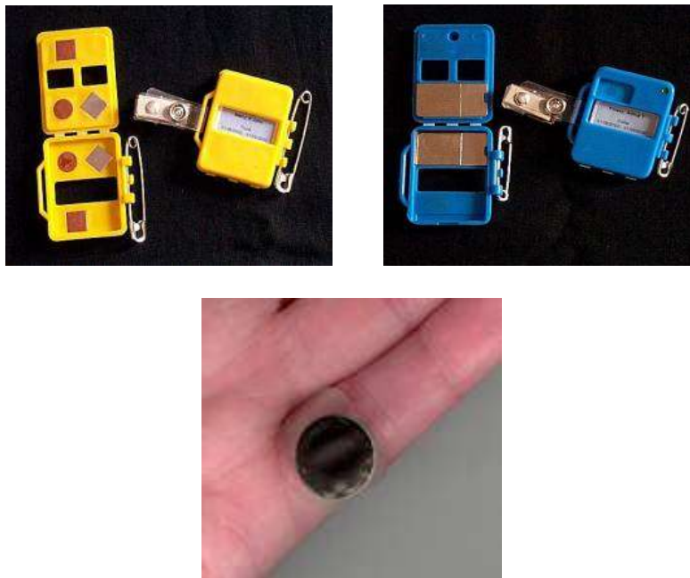
Fig 11 Examples of film badges and TLD ring dosimeters as used in NZ.
