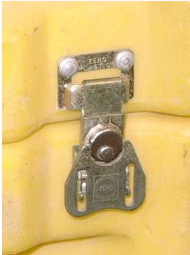
Fig 29 When the gauge is unattended it should be locked in its type A package/storage package. Most locks on these packages allow you to use a padlock or have key locks built in to them
