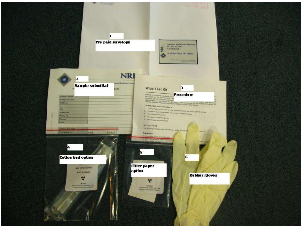
Fig 26 Example of a wipe test kit. This standard kit consists of the following items:
