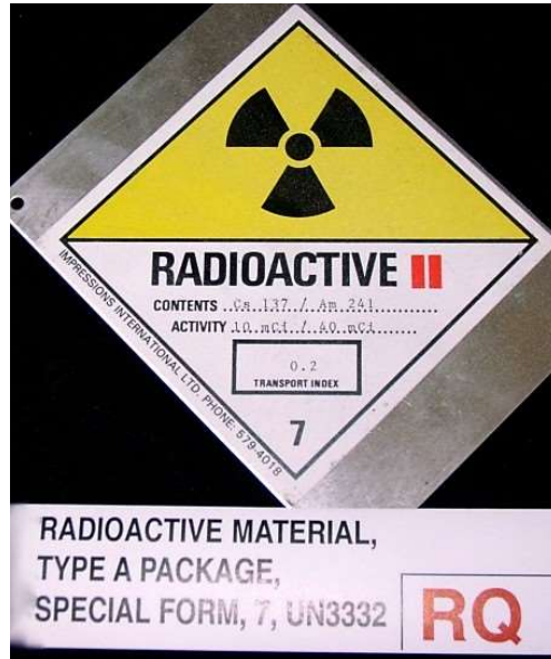
Fig 29 Current labelling requirements for the NDM. Note the UN number, transport index and contents
